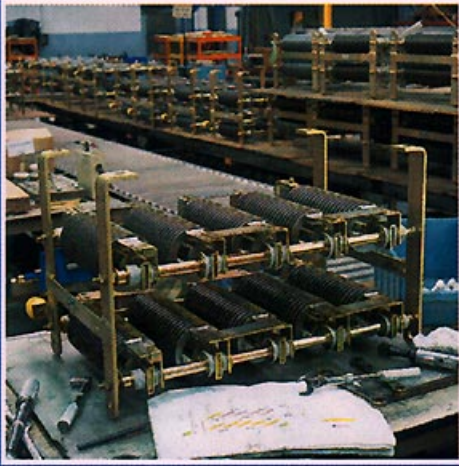
Fully assembled Resistor Banks ready for installation onto mounting rail.
