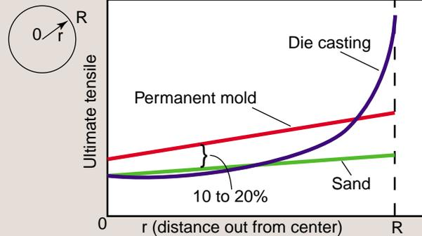
Permanent-mold castings cool faster than sand castings, giving them a much finer, more uniform microstructure. This boosts mechanical properties by up to 20%. In comparison, pressure-die-cast parts have a much stronger skin, but weaker interior sections.
