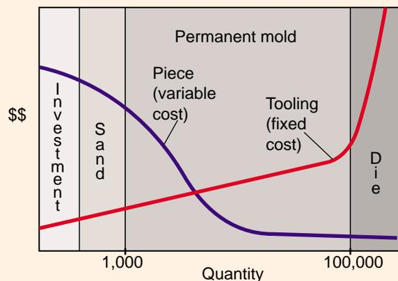
Sand casting involves temporary molds made from metal or wood patterns. Consequently, up-front investment for tooling is low, but per-part prices are usually higher than permanent-mold castings. Conversely, pressure-die casting has shorter cycle times which lower the per-part price, but tooling can cost up to 10 times that of permanent-mold tooling.
