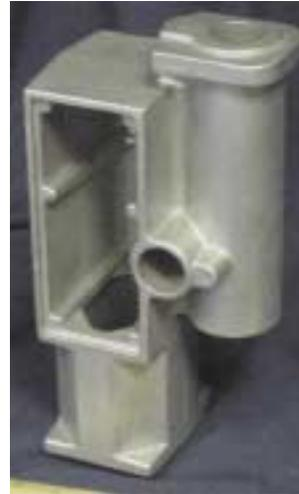
This housing for a heavy-duty portable magnetic drill weighs 7.16 lb and is highly cored to reduce the material removed during secondary machining.
