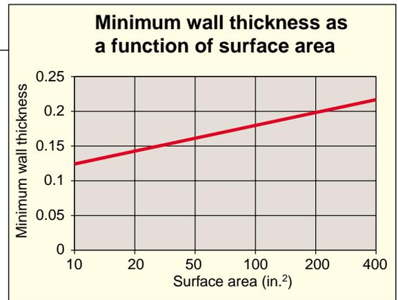
eas of the bottom as well as the four walls. This can be calculated and verified to be 180 in.<sup>2</sup> From the graph, the minimal wall thickness must be no less than 0.2 in. This tells us that our 0.25-in. wall thickness should be manufacturable. These values are minimums, however, and premised on a flat plate. As part complexity increases, so should minimum wall thickness.
