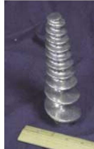
Permanent-mold casting is said to easily mold this complicated double helix, 83-lb auger mechanism for a juicing machine. Secondary finishing gives the auger its bright luster.
